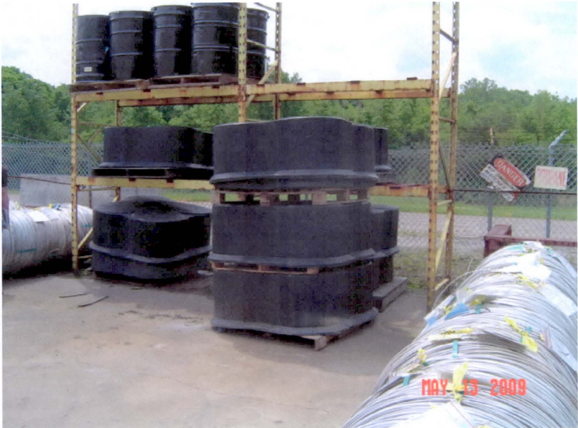
PHOTO #1 Special Metals -Rear Pad Hazardous Waste Storage Area -No adequate aisle spacing
