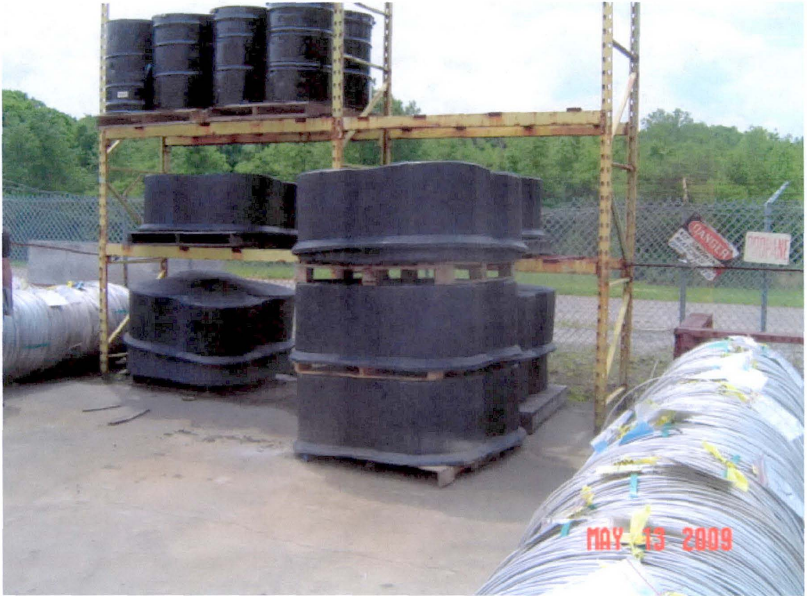
Special Metals -Rear Pad Hazardous Waste Storage Area -No adequate aisle spacing
