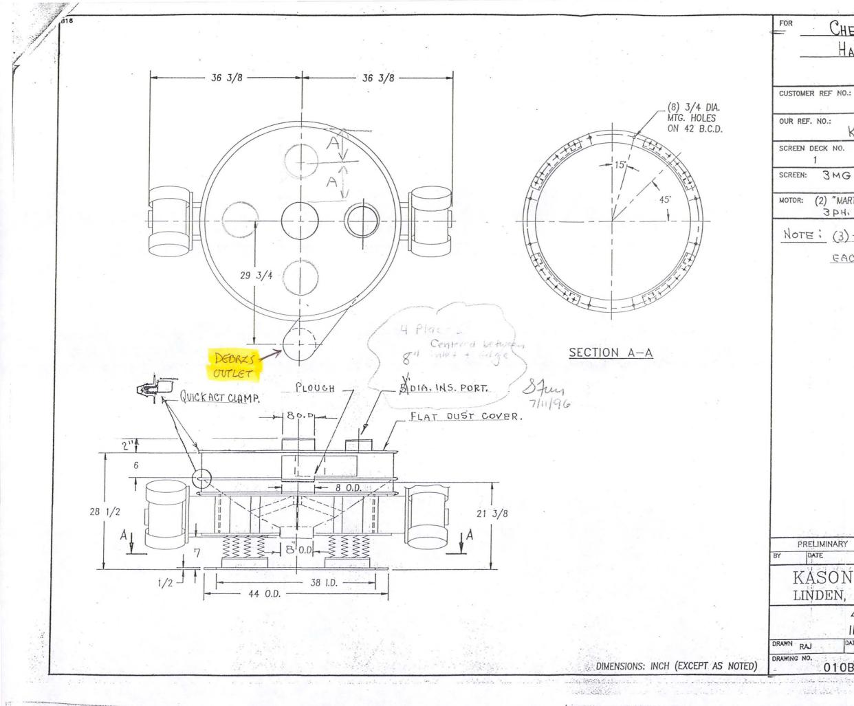
CHEMICAL SPECIALTIES HARRISBURG, NC. P.0.# A 1258 MODEL NO .: K-46610 K48-1FT- 55 NET WEIGHT FRAME NO. 900 LB 2 3MG(SS) MOTOR: (2) "MARTIN" CD12-1980, 11/16 HP.; 230/460V.; 3 PH.; 60HZ.; 1200 RPM, TENV. NOTE: (3) - 8 DIA, × 12 LG FLEX. CONN'R'S (WHITE NEO) EACH WITH (2) - (SS) CLAMPS ARE INCLUDED.
