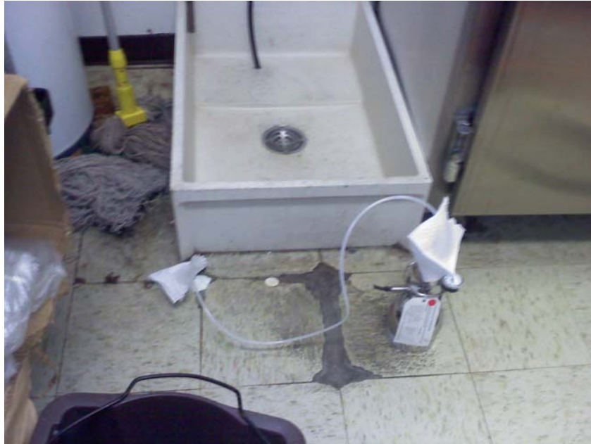
DSCA #01-0003 The sub-slab sampling location.
