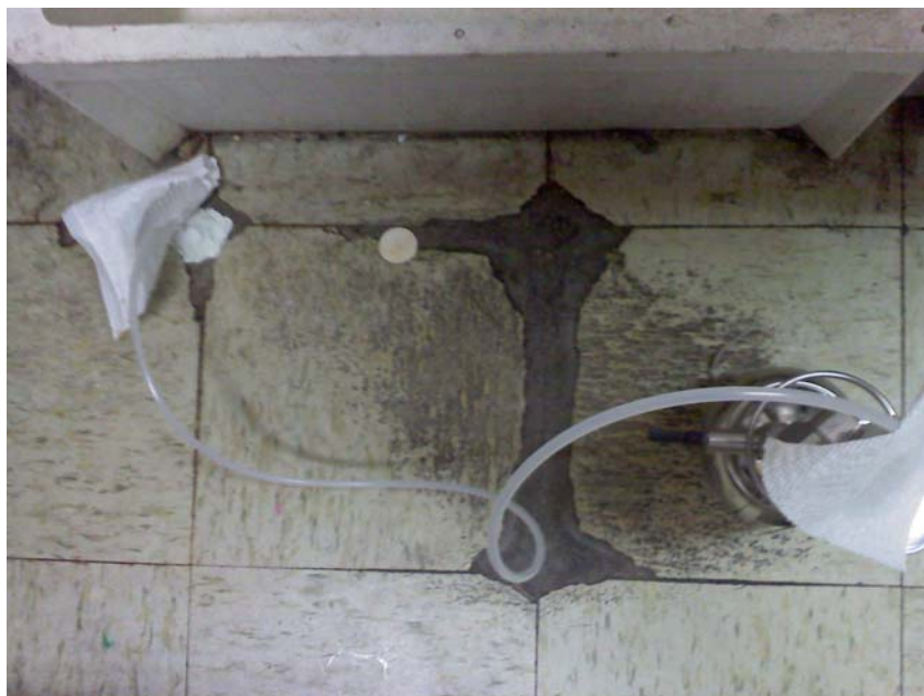
DSCA #01-0003 The sub-slab sample was collected in a one liter summa canister.
