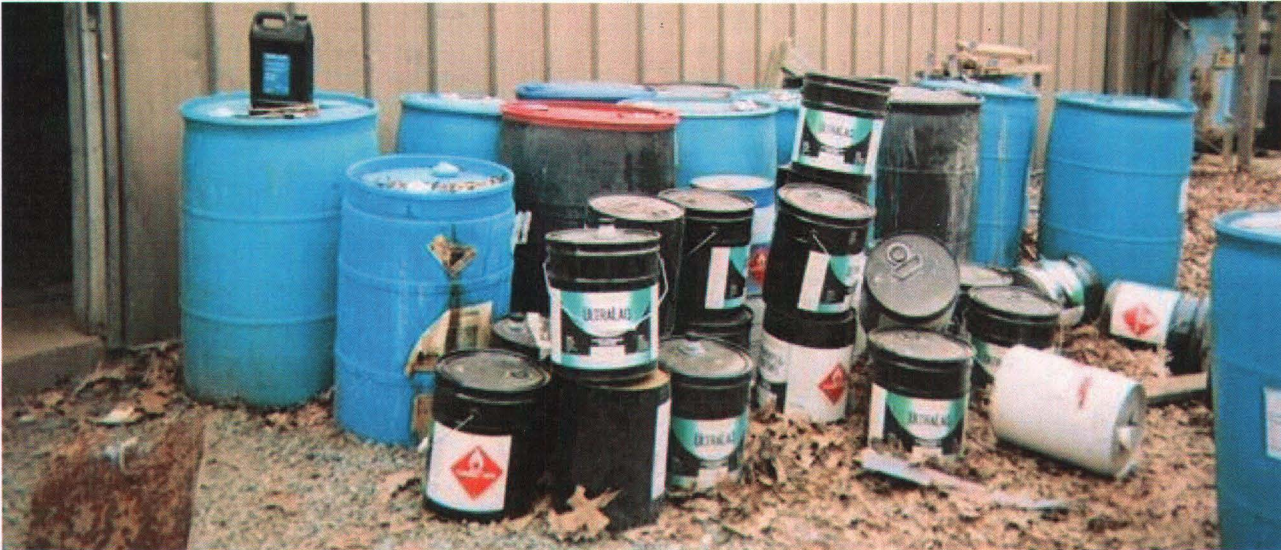
180-day hazardous waste storage area located behind Mumford Restoration contained seven 55-gallon drums and two 30-gallon drums of liquid hazardous waste (D001; F002-methylene chloride; F003-methanol; F005-toluene). None of the containers of hazardous waste were labeled or dated. Six of the containers were not closed. Inadequate aisle space was maintained (less than the required minimum of two feet) in the storage area. (Note: all of the small 5-gallon containers in front of the larger drums were empty as well as some of the larger drums).
