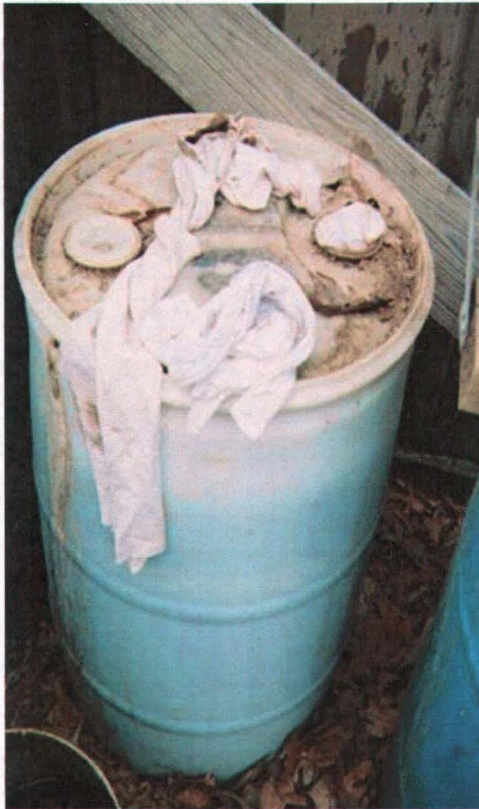
One 30-gallon open drum of liquid hazardous waste (D001; F002-methylene chloride; F003-methanol; F005-toluene) which was not labeled or dated was located in the hazardous waste storage area.
