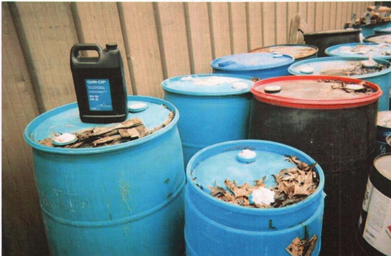
180-day hazardous waste storage area showing open containers of hazardous waste (D001; F002-methylene chloride; F003-methanol; F005-toluene). Rags were stuffed in the bung holes of the containers rather than utilizing appropriate container caps. None of the hazardous waste containers were labeled "Hazardous Waste" or marked with an accumulation start date. The facility did not maintain aisle space of at least two feet.
