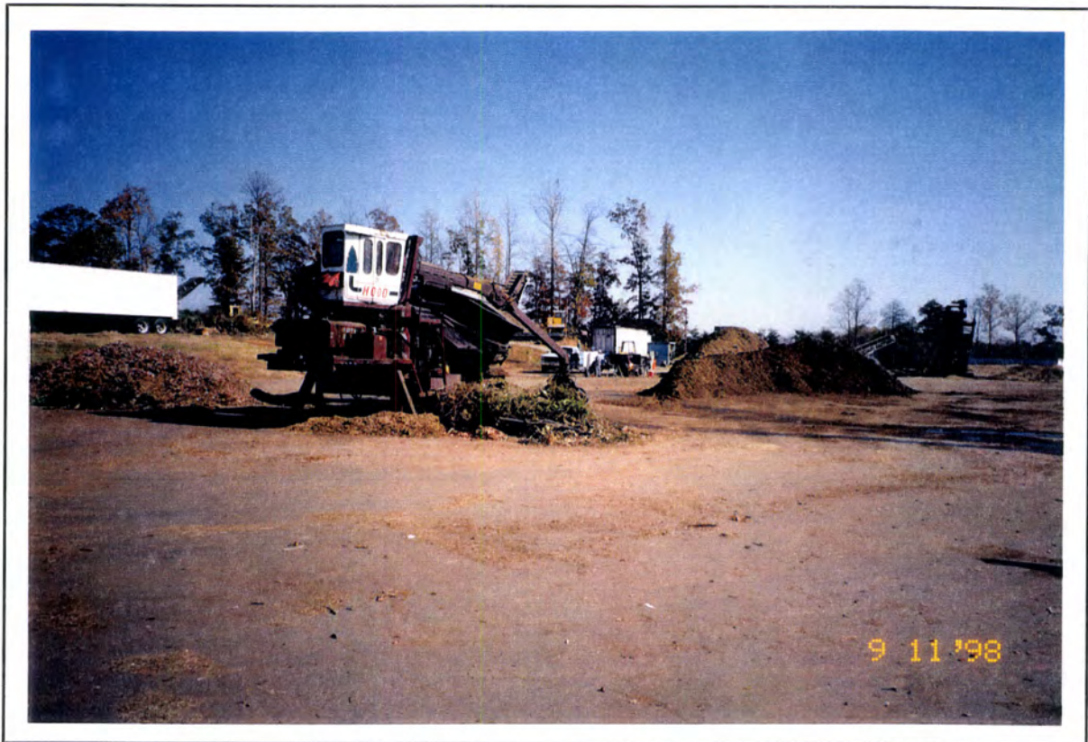
Portable Tub Grinder used for processing grass and leaves.
